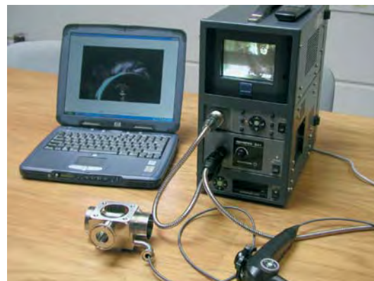
Boroscope inspection of the interior surface and weld seams of valves for aseptic applications
