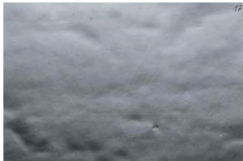
Microscopic view of mechanically polished and electro polished Ra 0,25 \mu\text{m} / 10 \mu\text{-inch}
