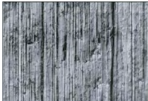
Microscopic view of mechanically polished surface with grit 400 Ra 0,25 \mu\text{m} / 10 \mu\text{-inch}
