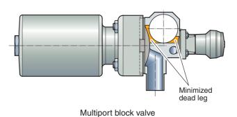
The complete drainability is an important consideration for the design of multiport valves. The following illustration shows the correct and incorrect installation of a standard T-valve:
